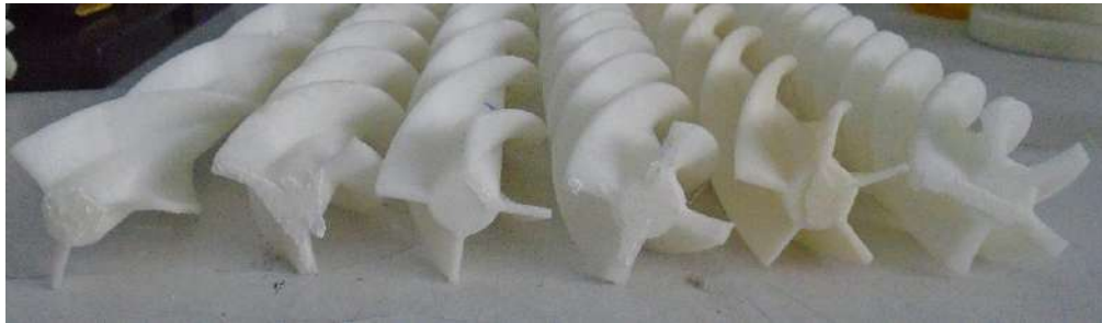
Figure 4. Helical baffles with 3,4 y 5 spirals to 45, 60 y 75 degrees of inclination.
