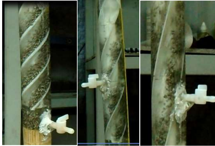
Figure 5. Baffle with 3 starts (from left to right) at 45 °, 60 ° and 75 °.
