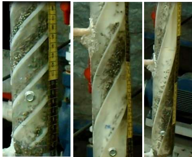
Figure 6. Baffle with 4 starts (from left to right) at 45 °, 60 ° and 75 °.
