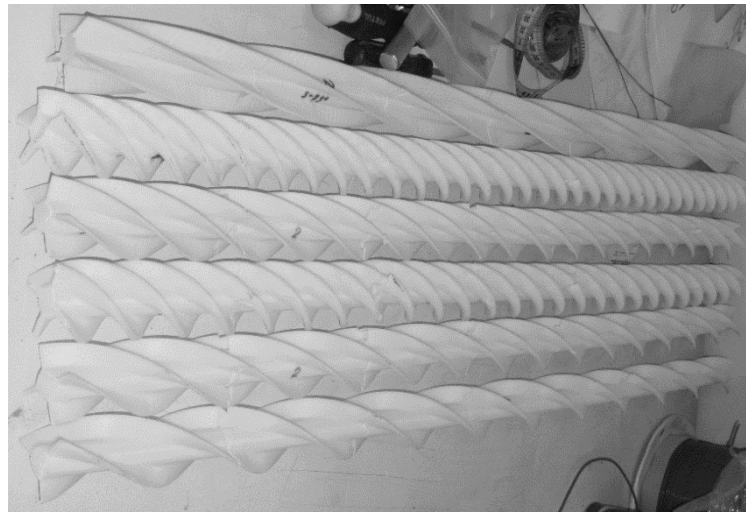
Figure 7. Helical baffles used in the experiments.
